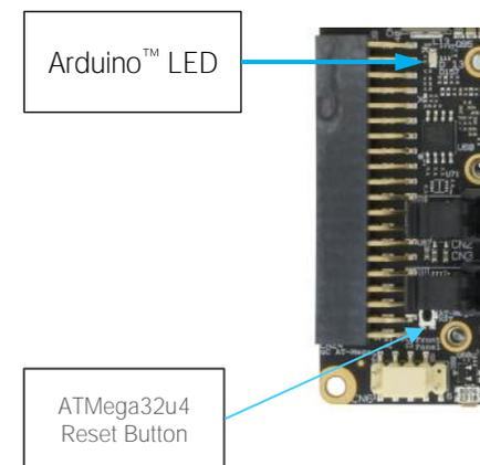
On-board, between the Arduino™ interface connector CN24 and the buttons/led header CN6, it is also available a miniaturized momentary switch, that can be used to reset the ATmega32u4 microcontroller.
