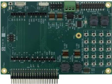
As a separated accessory, it is available an I/O Expansion board, which can be plugged directly on UDOO BOLT connectors CN24 and CN25, which will offer the interfaces described below.
