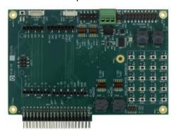
As a separated accessory, it is available an I/O Expansion board, which can be plugged directly on UDOO BOLT connectors CN24 and CN25, which will offer the interfaces described below.
