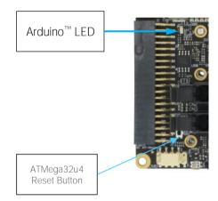
On-board, between the Arduino™ interface connector CN24 and the buttons/led header CN6, it is also available a miniaturized momentary switch, that can be used to reset the ATmega32u4 microcontroller.
